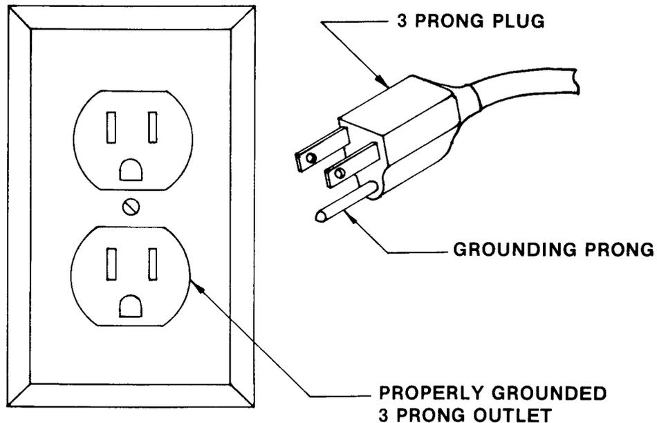
Plug power cord into 120V properly grounded type outlet protected by a 15-amp. time delay or circuit-saver fuse or circuit breaker.
